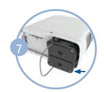
Remove the columns completely from the Inogen One® G<sub>5</sub>. Both columns are removed as one piece.
