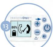
Press the alert/bell button once and screen will display "sieve reset success." Press the power button to turn on the Inogen One® G5, and use normally.
